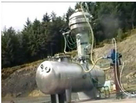
Full scale testing of a chemical reactor to establish its mechanical integrity during an internal explosion
